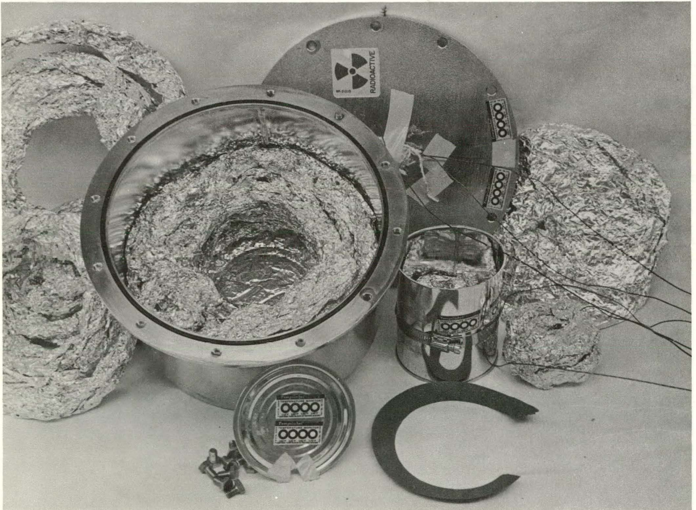
Figure 5. Inner Container and Lid, Food Can, Heating Element, and Metal-Foil Packing.
