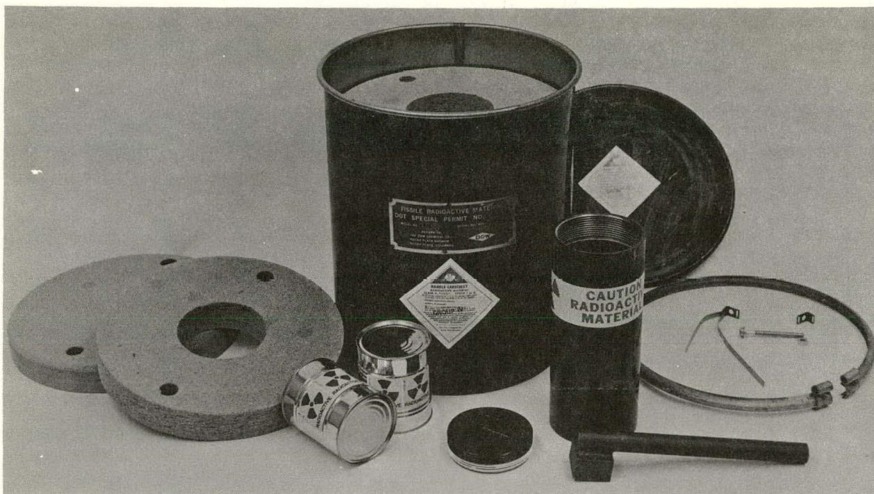
Figure 1. Model 1518 (DOT-6M) Container Showing Components and Sealed Food Cans Containing Plutonium Buttons.
