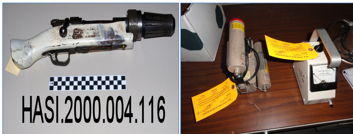
Fig. 4. Representative Artifacts from the Hanford Site: Left – A “Flange Gun” Modified on the Hanford Site to Produce a Flange on the End of a Reactor Pile Process Tube. Right – Radiation Detection Instruments including a “Hot Dog” Probe on the Left and a “Cutie Pie” Probe on the Right.
