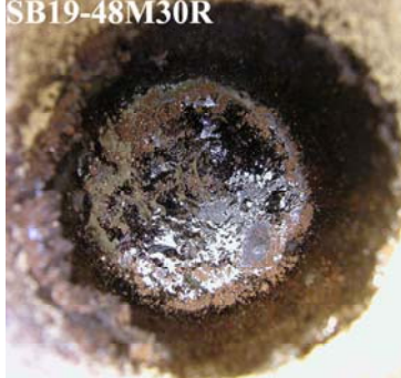
Figure 3.1. Top views of the melter feed blends after VGF experiments (30 and 60 minutes) with VS3 frit and SB19 simulant.
