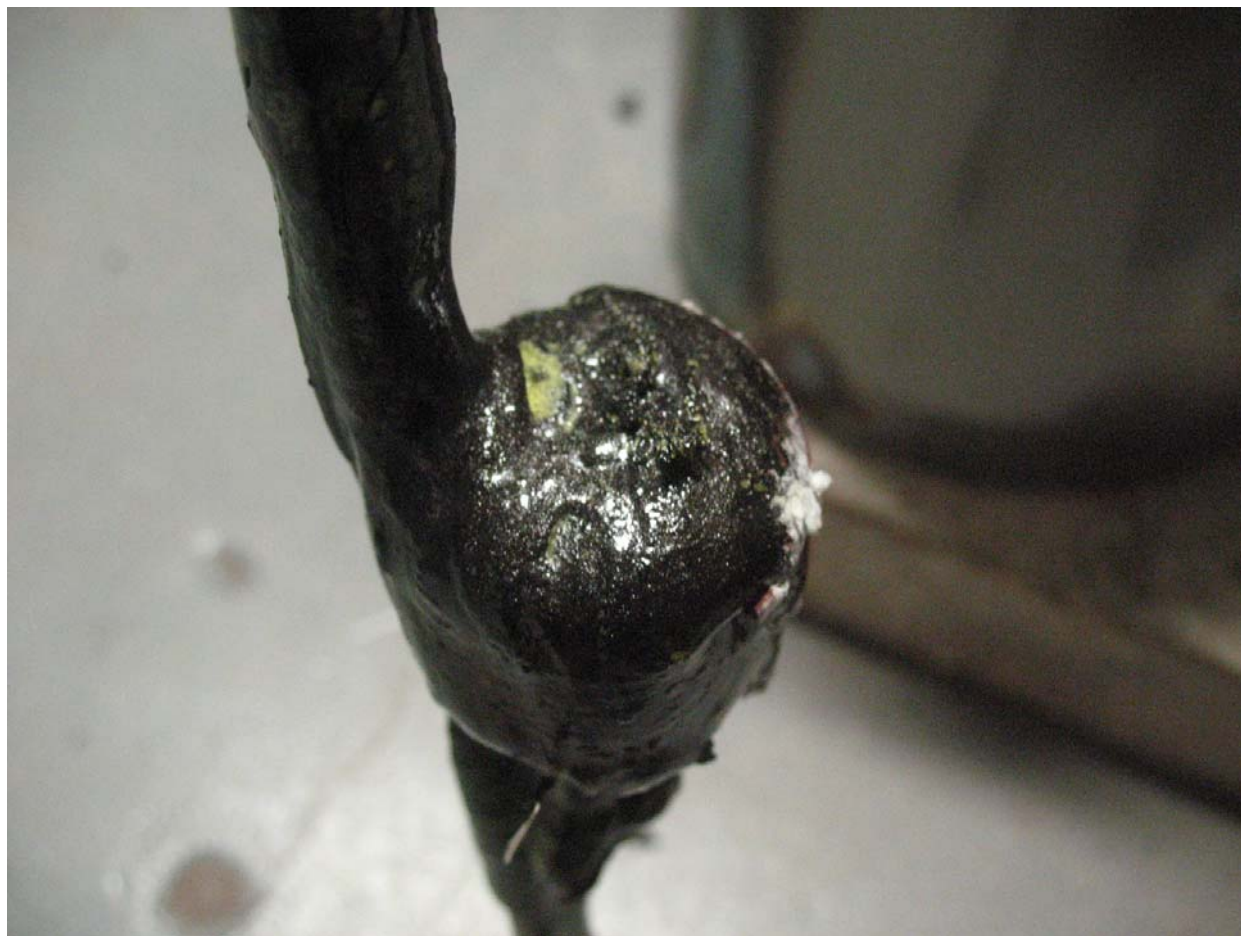
Figure 3.13. Upper sampling boat removed after Test 2 idling period. Note secondary sulfur phases on external glass surface.
