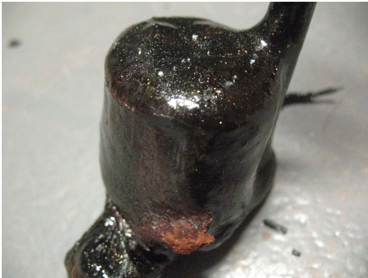
Figure 3.12. Lower sampling boat removed after Test 2 idling period.
