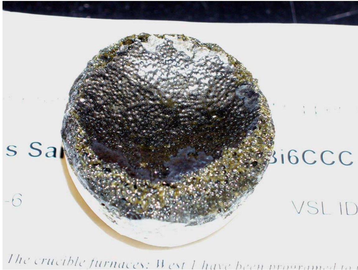
Figure 3.2. Top view of CCC sample of HLW-E-Bi6. Foaming observed is concentrated near the top of the sample.
