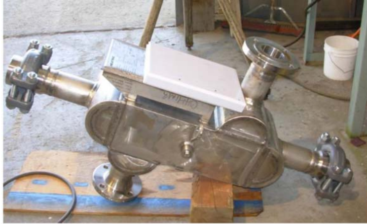
Figure 6: Printed Circuit Heat Exchanger from Heatric. This is a water to CO 2 heat exchanger sized for 0.51 MW th .
