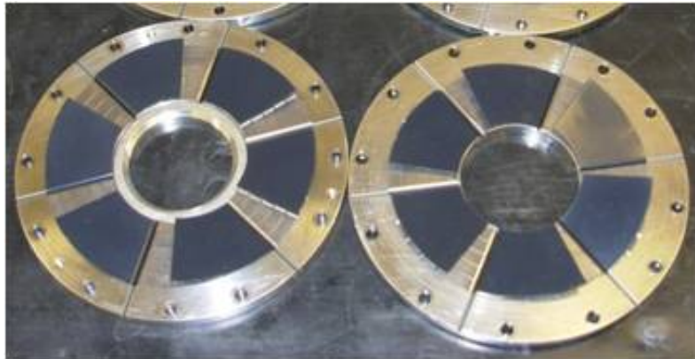
Figure 5: Gas-Foil Bearings used in the 1 MW th S-CO 2 Brayton Cycle at Sandia National Laboratories. For a commercial-sized unit, these bearings would be replaced with more appropriate components.
