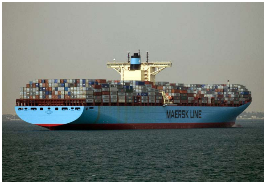
Figure 17. Container ship Edith Maersk, launched in 2007, displacement 170794 gross tons, length 397 m, beam 56 m, maximum speed 26 kts. (image courtesy Wikimedia Commons/Heb)
