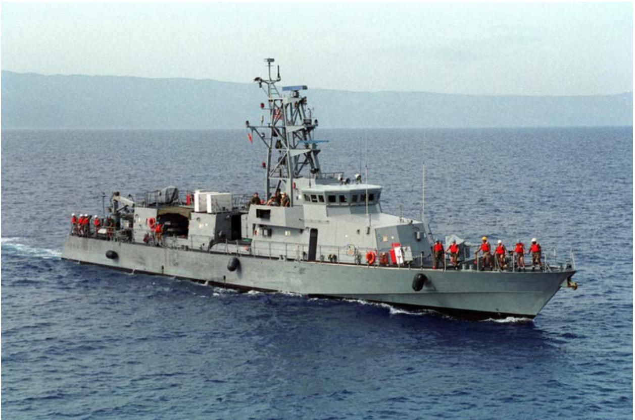
Figure 4. USS Tempest (PC-2) was the second Cyclone-class Patrol (coastal) ship, length 53 m, beam 7.6 m, maximum speed 32 kts. (image courtesy US Navy)
