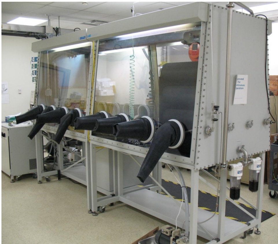
Figure 5: Argon-filled glovebox used for finished-material handling and testing preparation.
