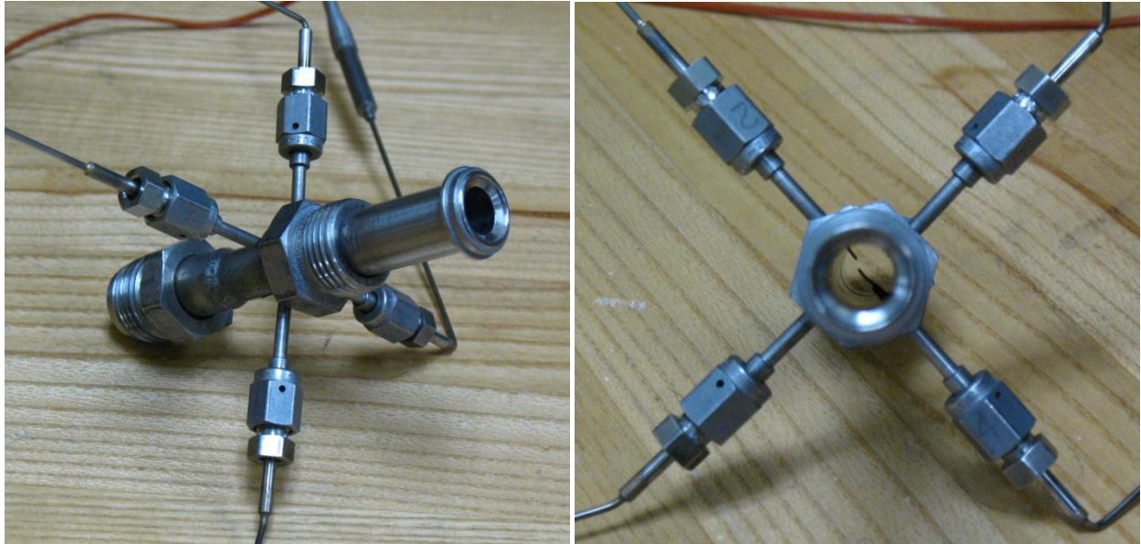
Figure 4: Sample holder for the flow-through calorimetry experiment. Axial view (right picture) shows the thermocouples that penetrate the sample to the center (from the bottom right) and to the midpoint radius (from the upper left). The other two thermocouples are flush with the sample holder inside wall.
