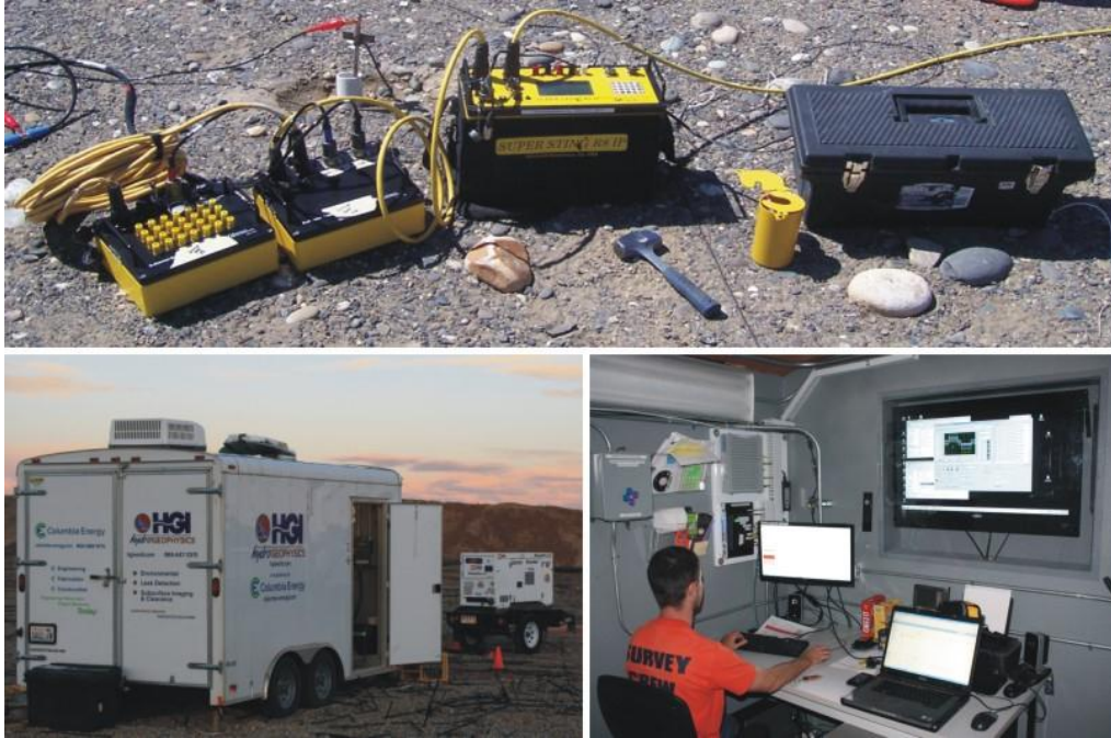
Figure 22. The SuperSting R8 Resistivity Meter (top) and Geotecton-180 Resistivity Monitoring System (bottom).
