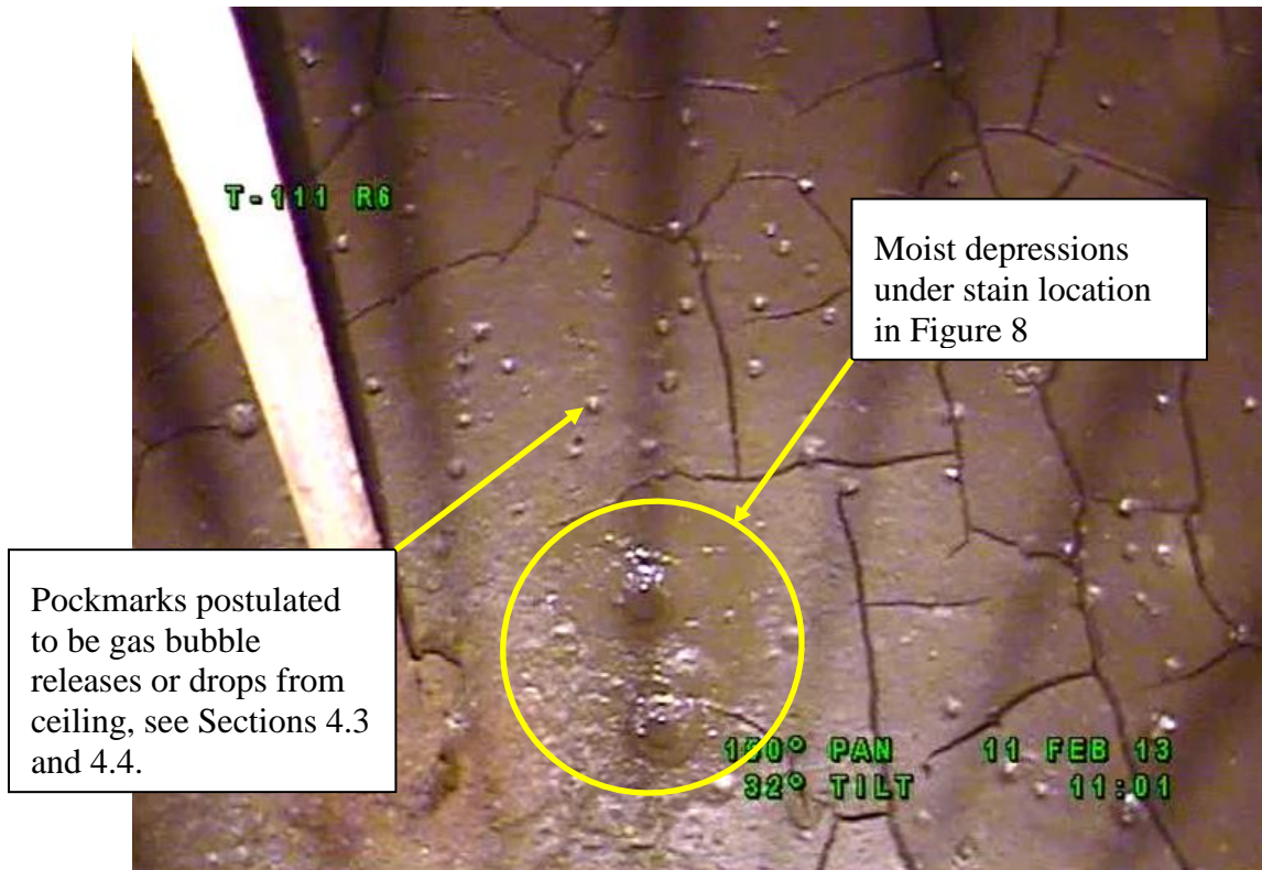
Figure 9 Anomaly on SE Area of Tank T-111 Dome Just Above Top Stiffener Ring
