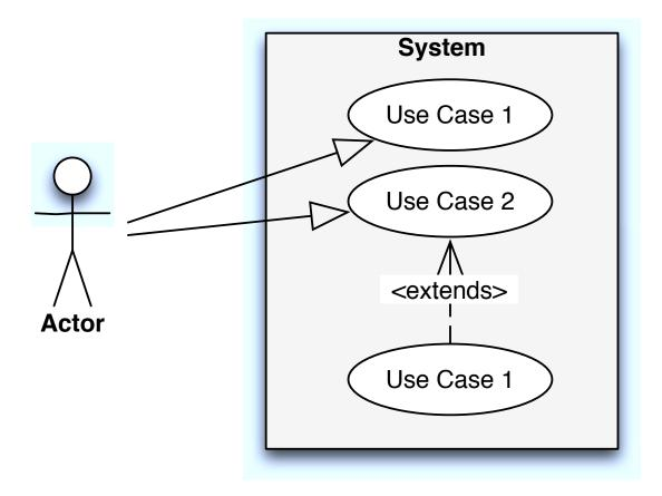
Figure 1. Example Use Case Diagram
