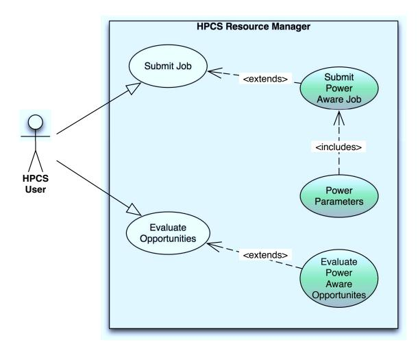
Figure 17. HPCS User  $\Rightarrow$  HPCS Resource Manager Use Case Diagram
