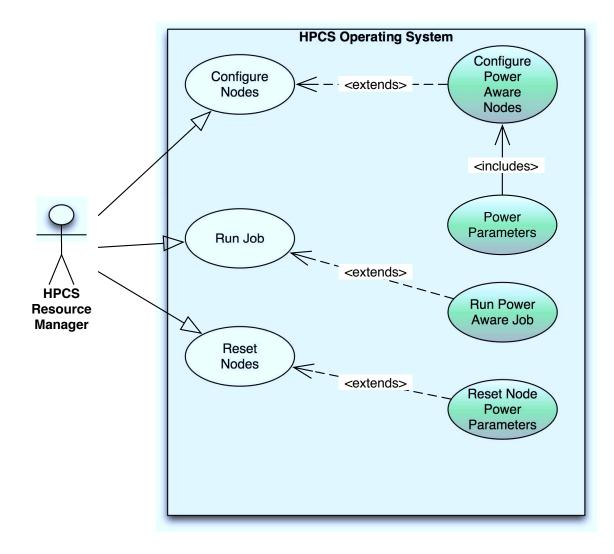
Figure 10. HPCS Resource Manager  $\Rightarrow$  HPCS Operating System Use Case Diagram
