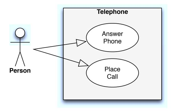
Figure 3. Person/Telephone UCD - Correct Level
