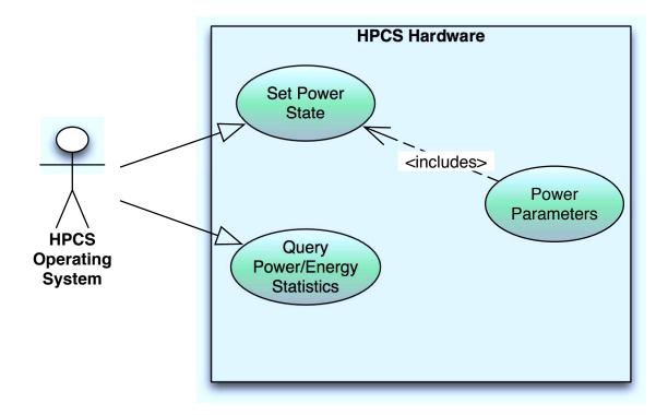
Figure 11. HPCS Operating System  $\Rightarrow$  HPCS Hardware Use Case Diagram
