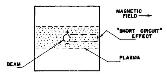
In an actual thermonuclear device the neutralizing plasma should have its greatest density near the center of the system. This plasma could be formed by various means such as PIG discharges, arcs, RF discharges, or perhaps by ionization of the residual gas by the incoming beam. The polarized beam passes through the magnetic field until it reaches a plasma region sufficiently dense to neutralize it at which point it is trapped.
