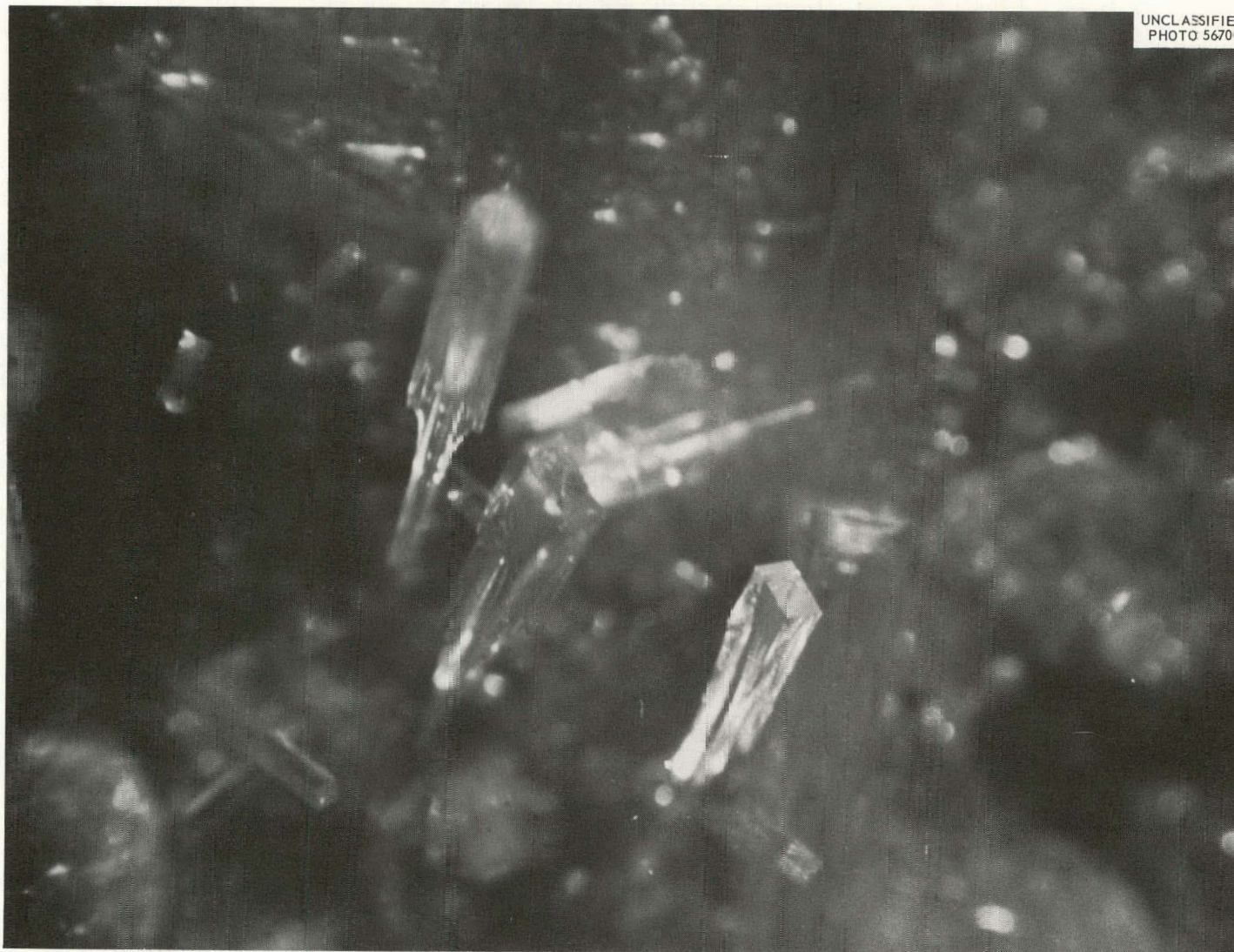
Fig. 5. LiF Crystals Grown from Vapor (in Place).
