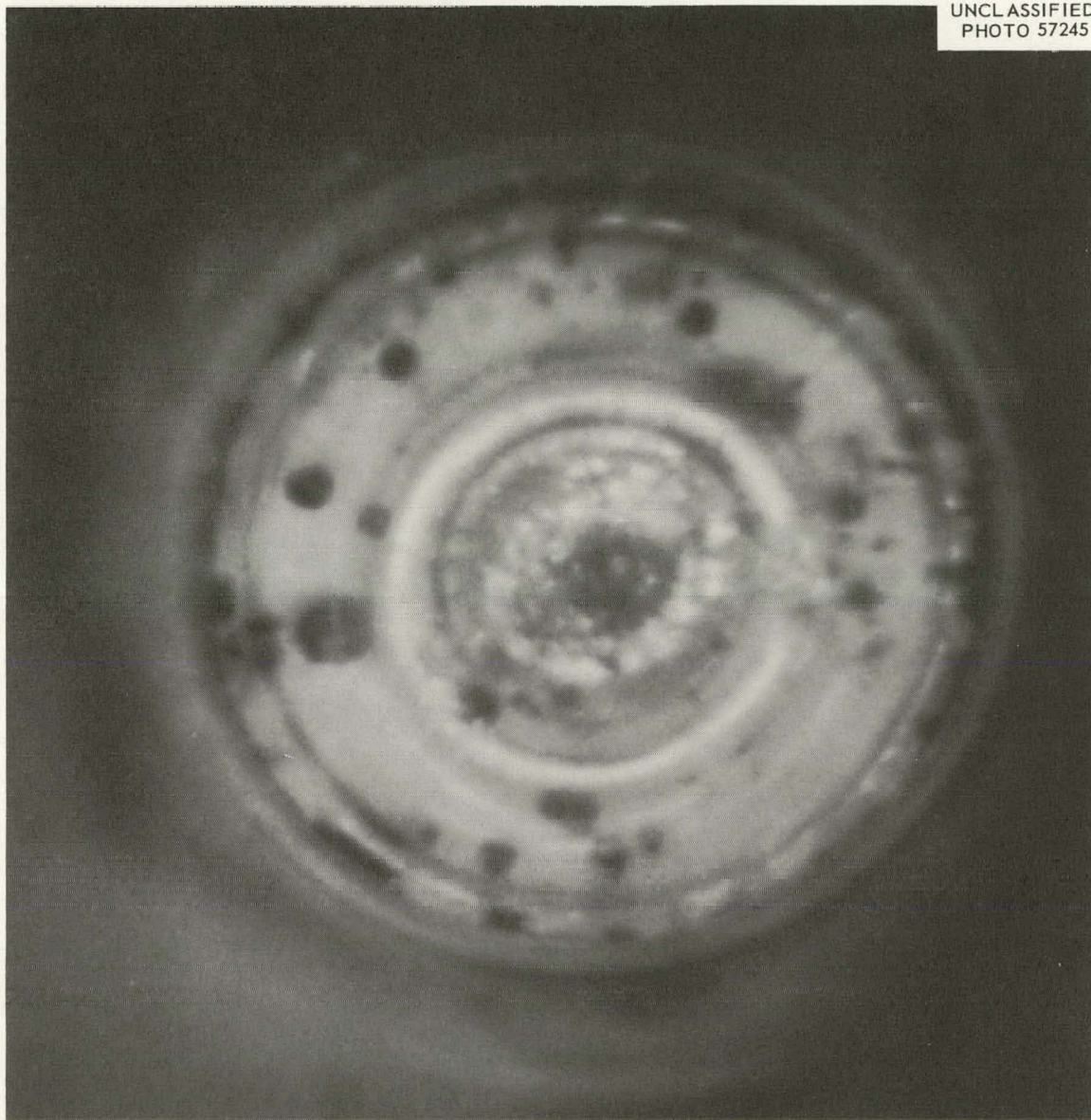
Fig. 9. Crystal at 830°C Viewed Through Quartz Window.
