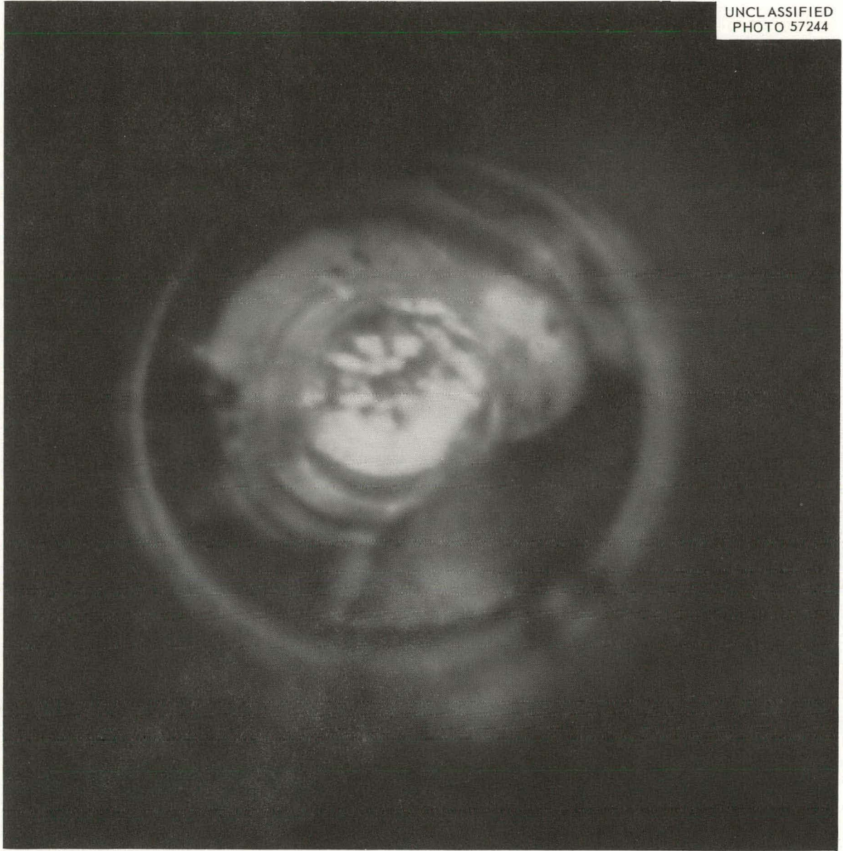
Fig. 8. Partly Sublimed LiF Charge at 830°C.
