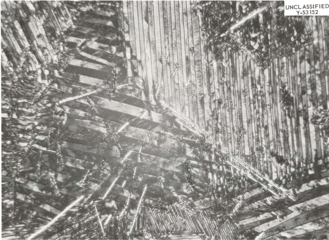
Fig. 2. Microstructure of Thorium Dicarbide under Polarized Light Showing Extensive Twinning and Massive Stringers of Graphite. 1000X.
