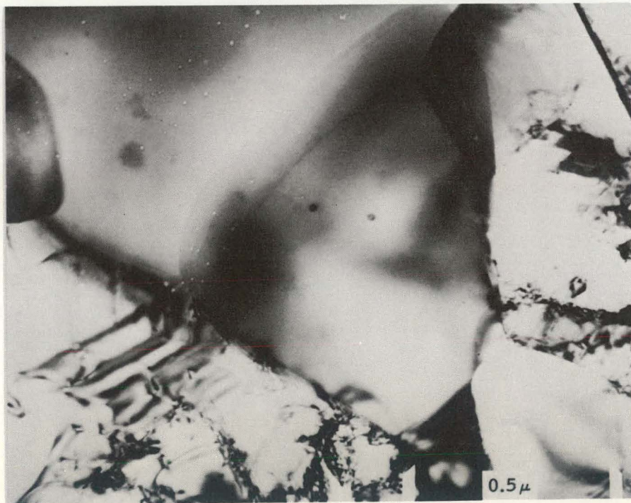
b. Transmission-Electron Micrograph Showing Helium Bubbles in the Ferrite Phase
