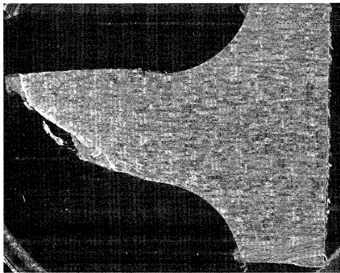
Figure 22. Microstructure of 1132 Sample Fatigued at 300°F [(Specimen II-2 (tested at 0.40% strain at 300°F... failed at 11,400 cycles). Unworked shoulder of the specimen appears unaffected by temperature. Worked portion in the gage length shows considerable grain refinement and reorientation. Some surface roughening occurred. Fracture is in maximum shear direction.] (~4X)
