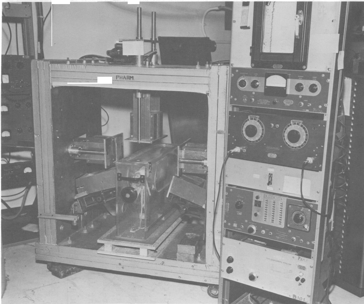
FIGURE 1.26. Whole Body Longitudinal Scanning System for Detecting Radionuclides in Dogs
