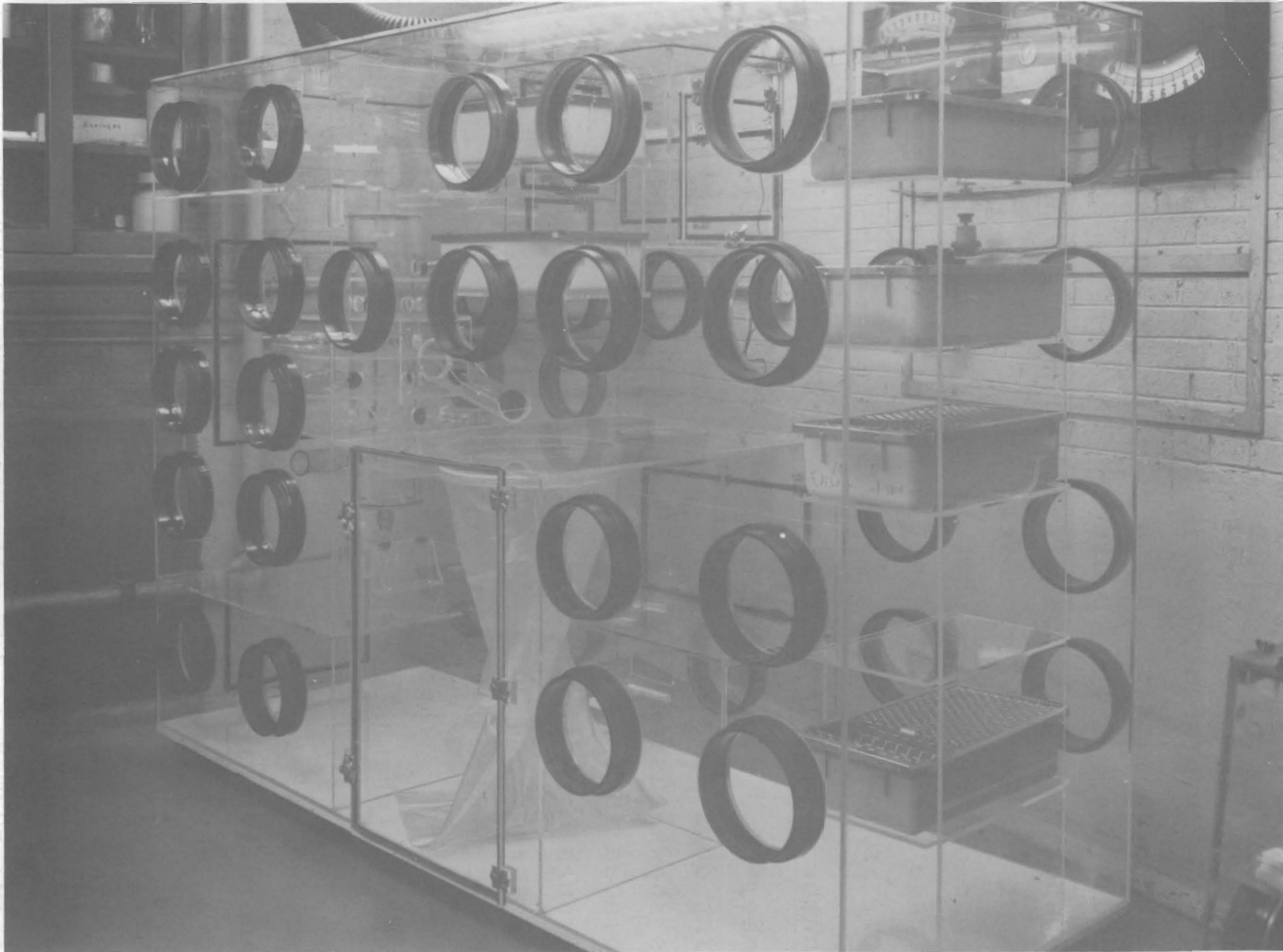
FIGURE 1.6. Multi-Compartment Glove Box Containing Aerosol Exposure Chamber, Cage Storage Area, Radioactive Waste Storage, and Aerosol Generators for High Level Radionuclide Exposures of Rats
