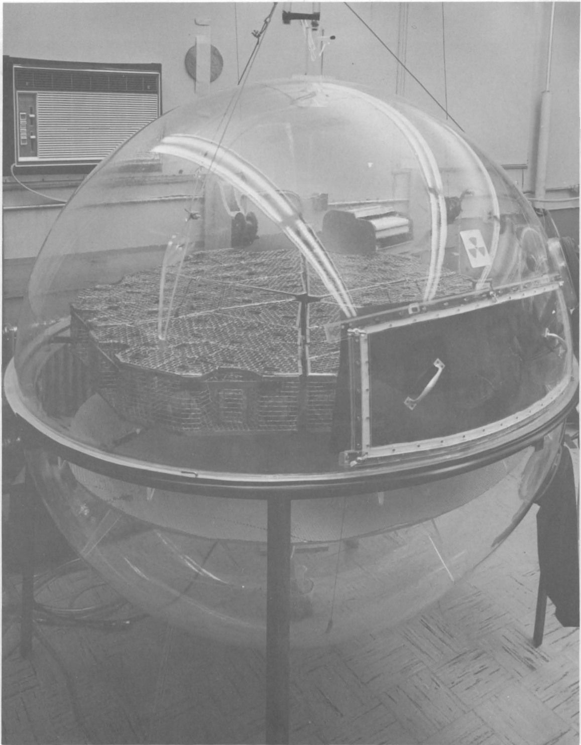
FIGURE 1.7. Spherical Aerosol Chamber for Daily Exposure of Hamsters to Constituents of Uranium Mine Environment
