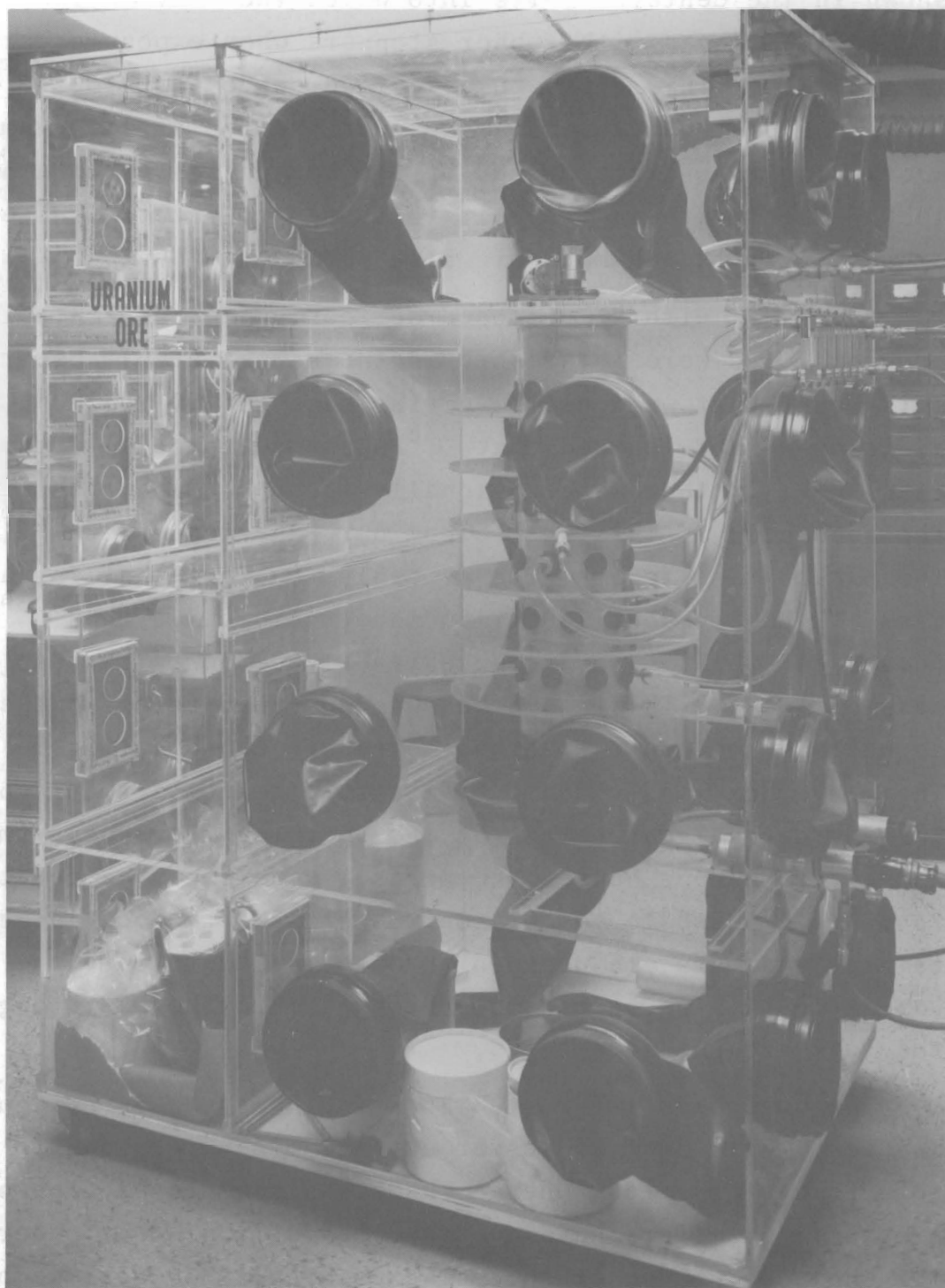
FIGURE 1.5. Glove Box Containing Aerosol Exposure Chamber and Cage Storage Space for Rats
