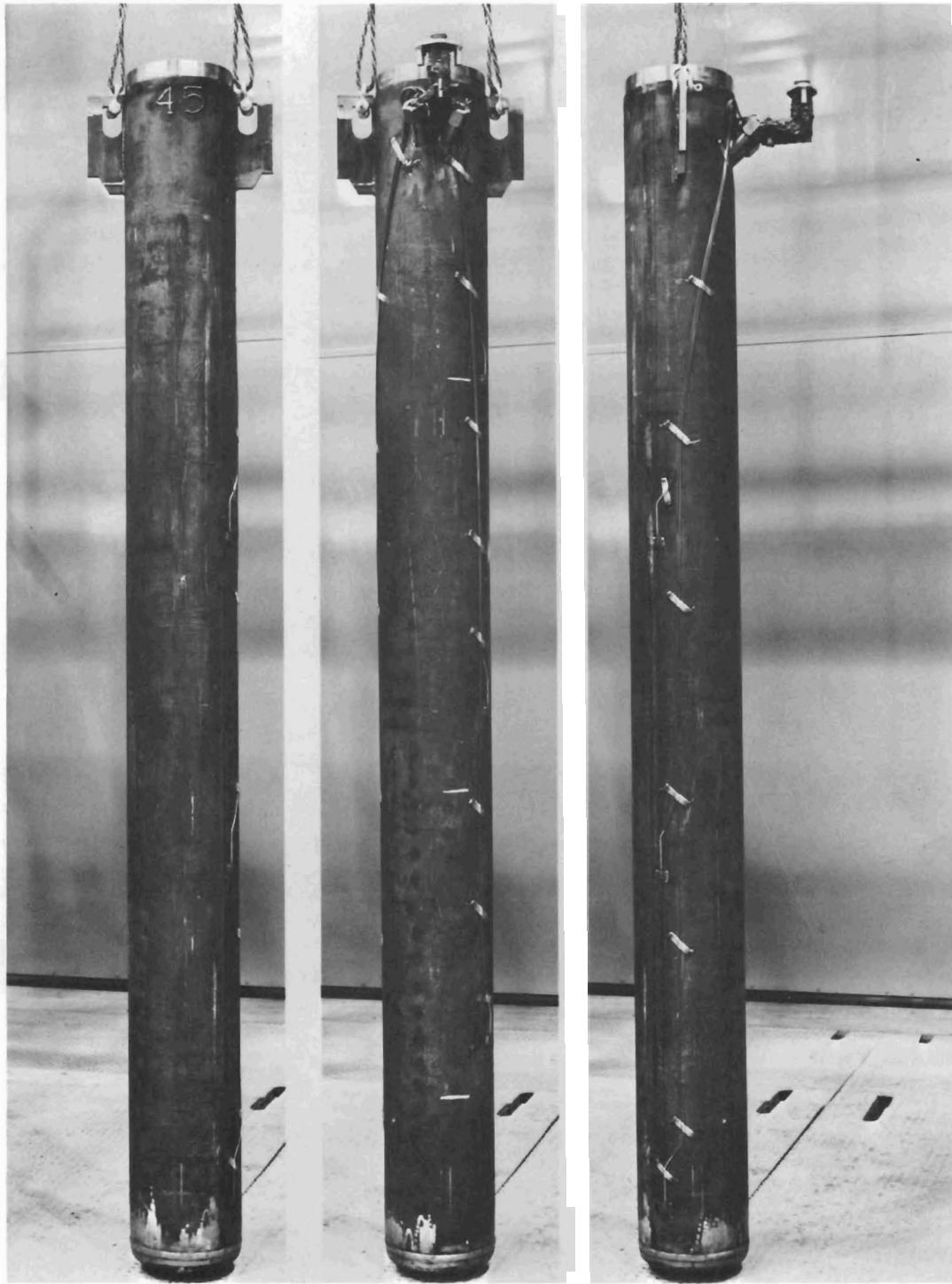
FIGURE 6.5. Phosphate Glass 8-Inch Waste Container (PG-11)
