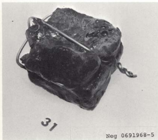
FIGURE 6.6. Thermal Shock Test Coupons for Spray Solid (PW-1 and PW-2)
