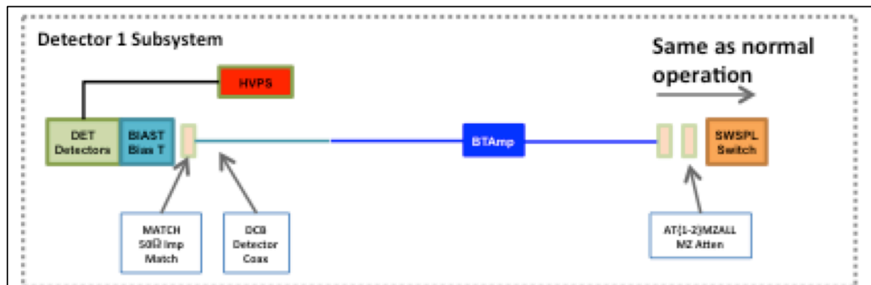
Figure 11. Schematic showing setup during amplifier use on a timing shot. Two 1.44m lengths of HF290 and the amplifier are added to the signal path (shown in dark blue).
