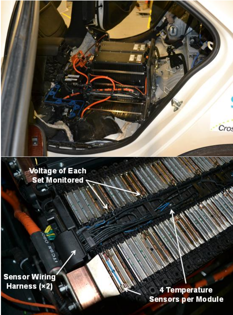
Figure 19 – As the project progresses, the team would like to install a full complement of LLNL-YTP wireless tags and sensors on the Colorado State University (CSU) plug-in hybrid-electric vehicle (PHEV) known as EcoCAR 2. This will enable Professor Bandhauer and his mechanical engineering students to further quantify tag performance in complex environments representative of state-of-the art PHEVs. Advantages of involving CSU include the opportunity to use these new wireless sensors and the more fully instrumented PHEV to educate next-generation energy engineers.
