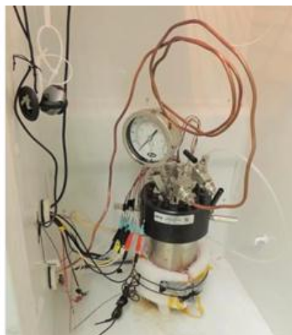
Argon-filled autoclave with copper tubing and electronic connections
