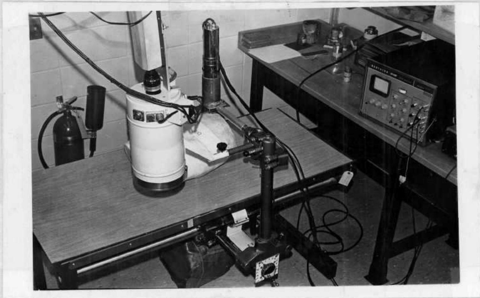
Figure 4: A photograph of the vertebral bone mineral measuring apparatus with the NaI(Tl) crystal and photomultiplier tube in position over a torso phantom. The white cylinder to the left is the image intensifier.
