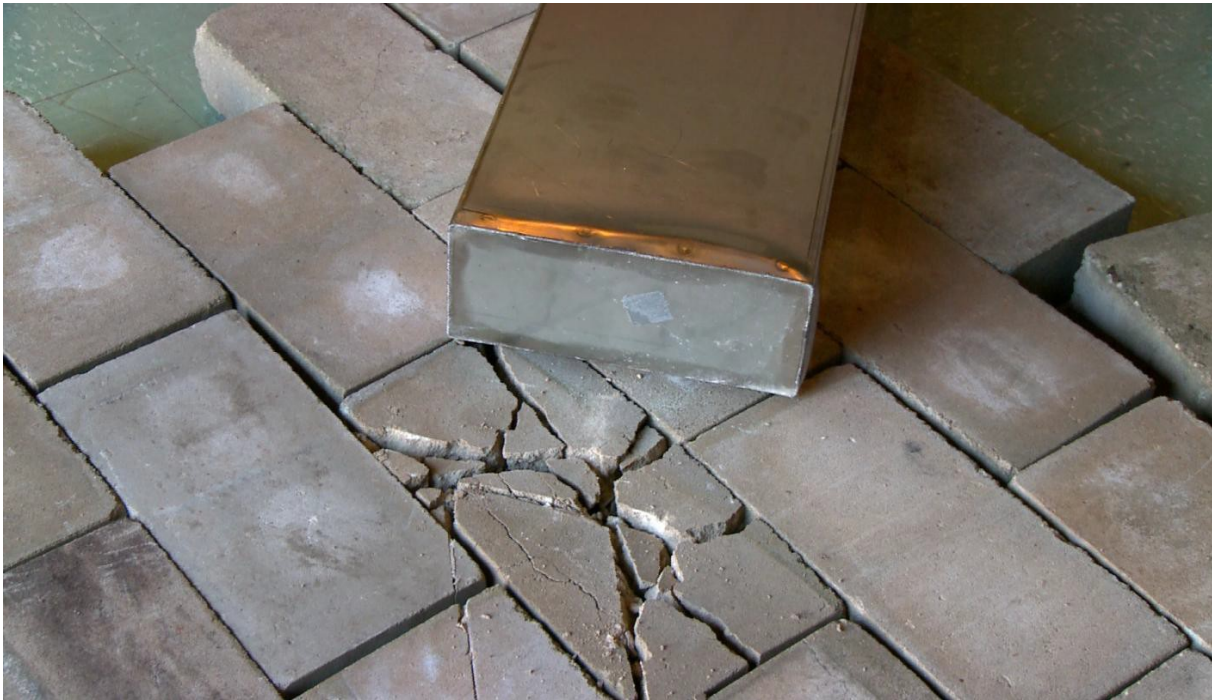
Figure 2: This photograph (after impact) depicts the damage to the concrete bricks and the damage to the stainless steel case for the detector assembly. The stainless steel case was not breached.
