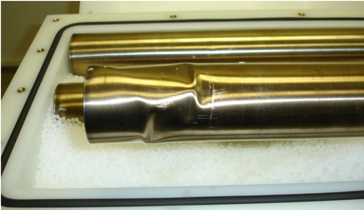
Figure 4: A close-up view of the most damaged tube from the drop test mock-up. While wrinkled, the tube has not been breached. The tube is being held above its installed position in the mockup for this photo.
