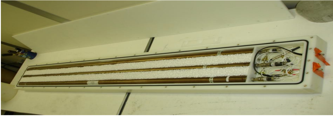
Figure 1: This is a photograph of the full assembly, showing the machined one-piece cavity with o-ring seal, the tubes with electronics modules, and the alumina and poly bead blend, just prior to assembly. The top cover can be seen leaning against the wall.
