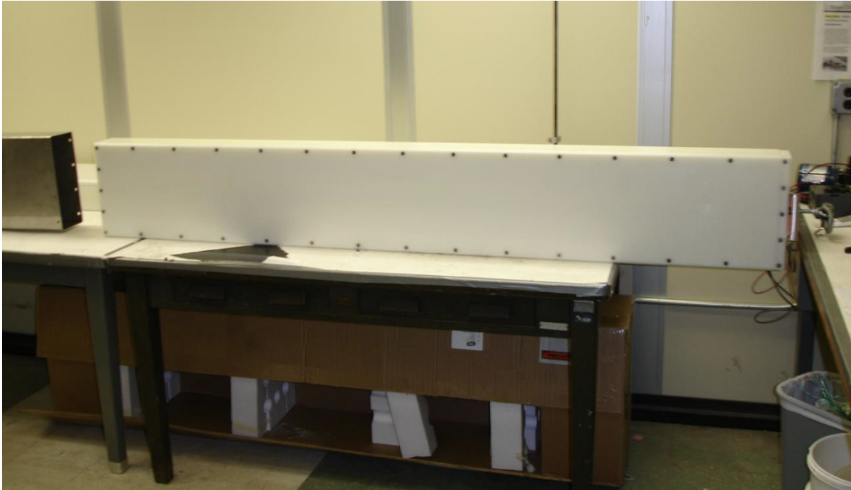
Figure 3: The polyethylene cavity after being slid out of the stainless steel envelope.
