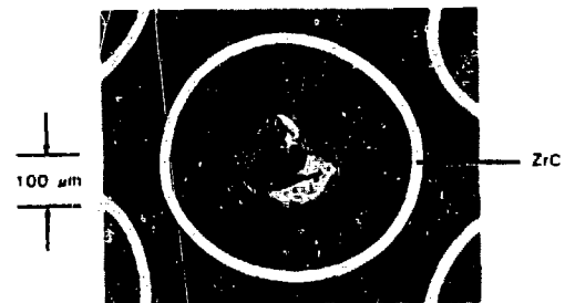
Fig. 7. Coated particle with graded C-ZrC-C alloy coat. The graded coats contain more than one hundred alloy compositions and appear continuous.
