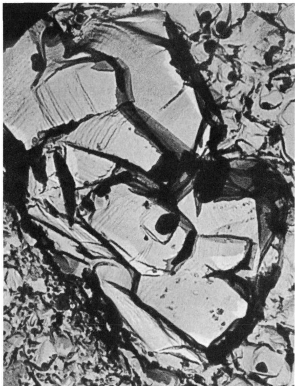
Figure 7. Carbon replica, pre-shadowed with Pt-Pd, of A255 alloy after corrosion for 12 min at 250°C.
