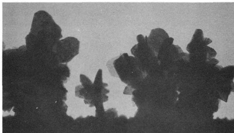
Figure 8. Carbon replica, pre-shadowed with Pt-Pd, of A255 alloy after corrosion for 12 min at 250°C.
