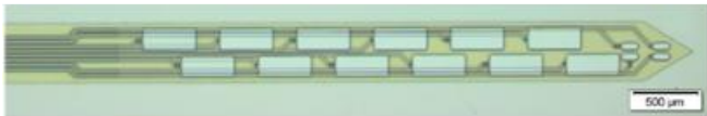
Figure 1. Image of the stimulating electrode array. The twelve stimulating electrodes are each 150 \mu\text{m} by 400 \mu\text{m} . The four small electrodes at the right of the probe are designed for future use as electrochemical sensors.
