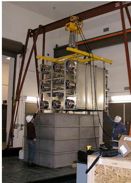
Figure 3: Assembly of the inner detector volume.
