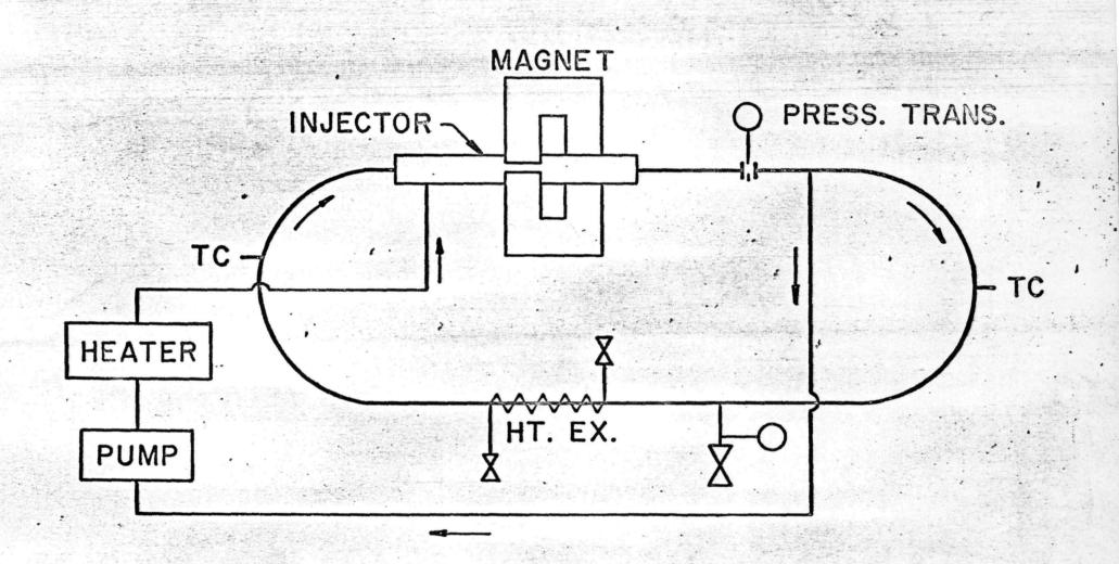
Schematic Diagram of MHD Circuit
