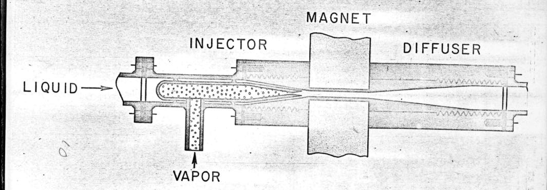
Cross Section of Jet Injector
