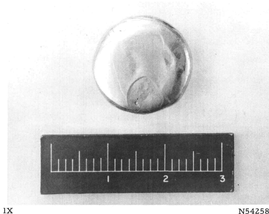
FIGURE 1. TYPICAL ARC-CAST 200-G BUTTON OF UNALLOYED TANTALUM
