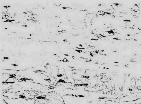
d. Nominal Iron-25 w/o Chromium-5 w/o Aluminum-1/2 w/o Niobium-1/2 w/o Titanium Alloy (Heat 53)
