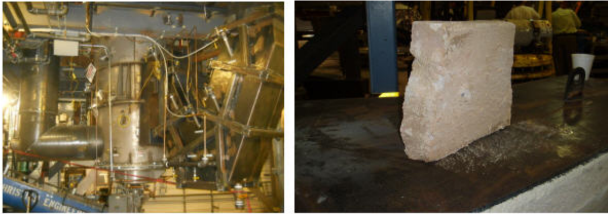
Figure B-3 – RBO (left) and the smaller of two refractory pieces removed from the RBO (right)
