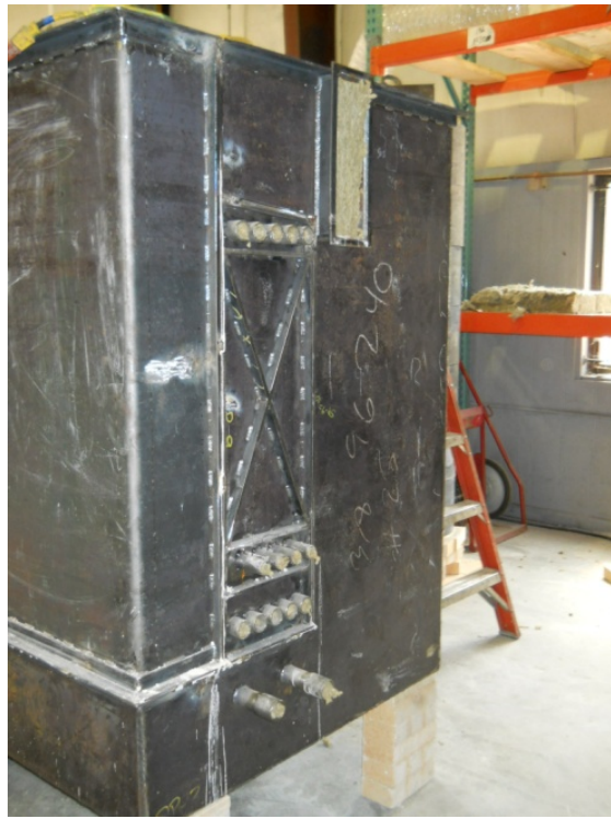
Figure 5-10 – Reducer main SPCV under construction
