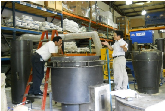
Figure 5-13 – Primary and Secondary Cyclones during fabrication
