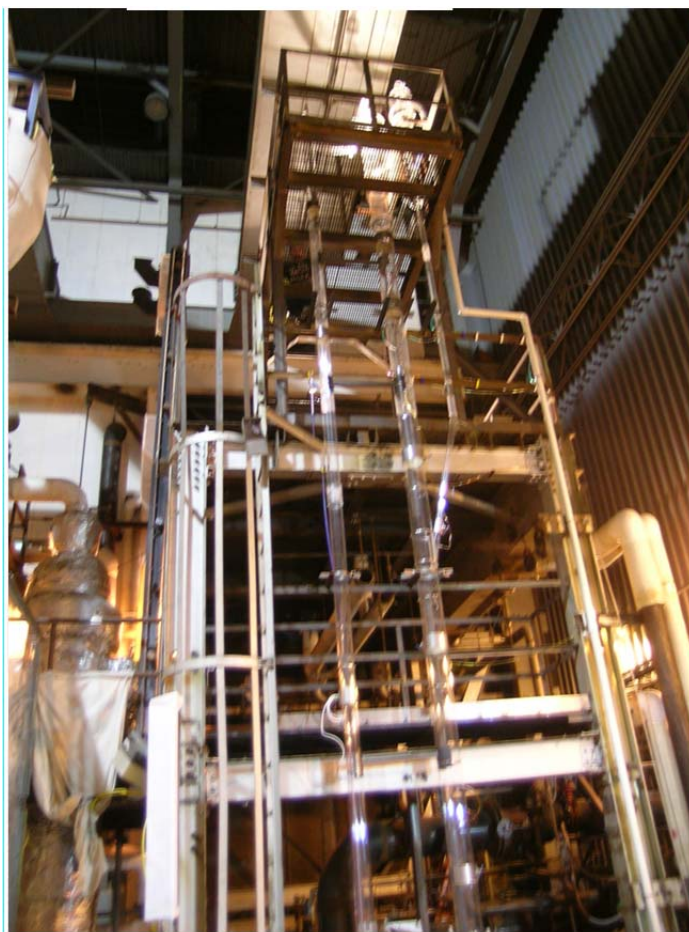
Figure 6-1 - 40 Foot Cold Flow Model with a 4" Riser
