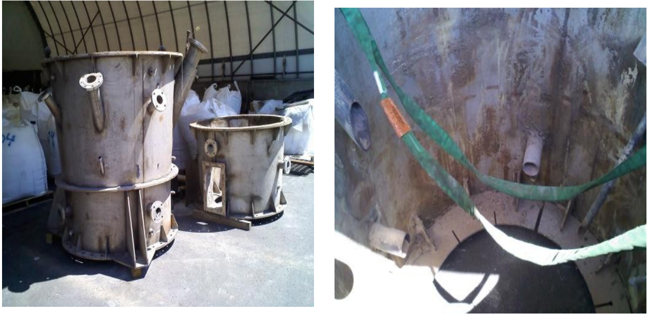
Figure 5-8 – Oxidizer before modification with refractory removed
