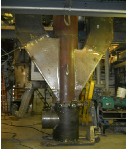
Figure 5-12a (left) – Cactus and Lower Reducer Figure 5-12b (right) – SPCVs and lower Reducer installed
