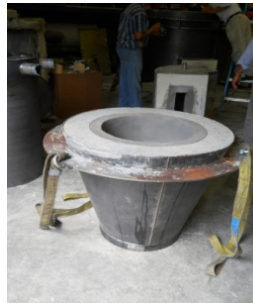
Figure 5-13 – Primary and Secondary Cyclones during fabrication
