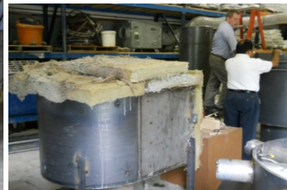
Figure 5-13 – Primary and Secondary Cyclones during fabrication
