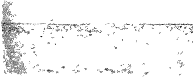
(A) Al/Ni HOT-PRESSED COUPLE. 12-tsi pressure, 500°C, HF etch- polish. 1000X.
