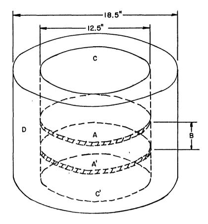
A and A'-Equal Thickness Plutonium Metal Slabs B-----Plexiglass Separation Thickness Cand C'--Plexiglass End Reflector 4 Inches Thick D-----Plexiglass Lateral Reflector 3 Inches Thick
