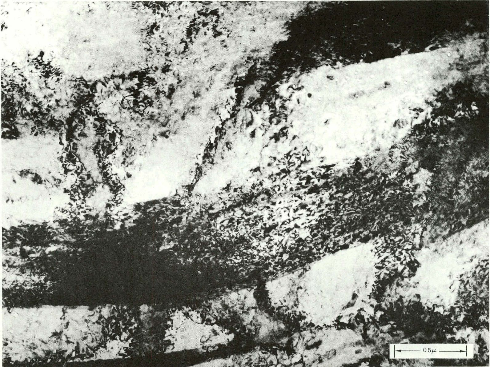
18-279 Figure 3. Microstructure of 20% Cold-Rolled Type 316 Stainless Steel after Irradiation at 500 to 530°C to a Fluence of 3.8 \times 10^{26} n/m 2 (E > 0.1 MeV)
