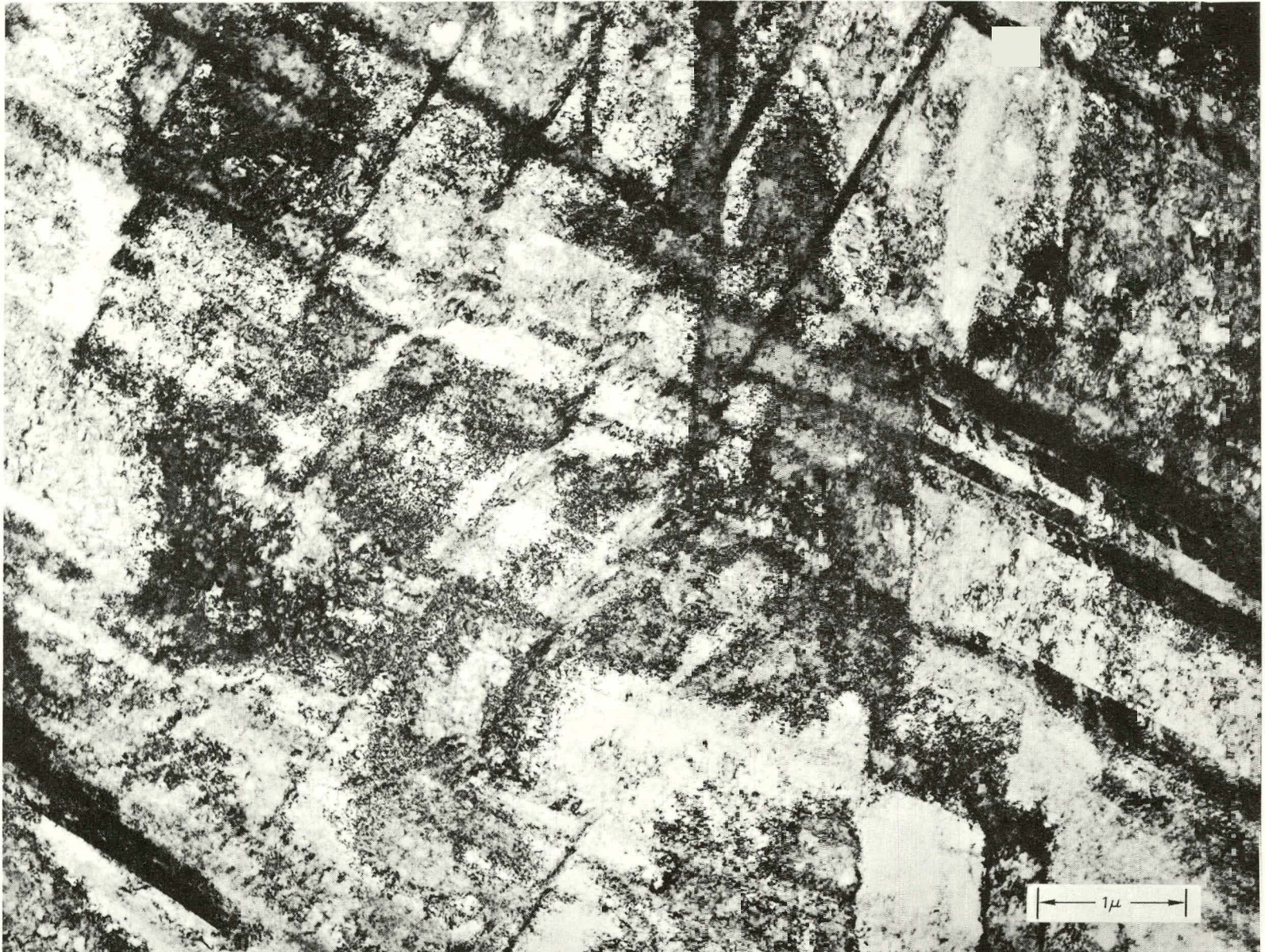
Figure 2. Pre-irradiation Microstructure of 20% Cold-Rolled Type 316 Stainless Steel
