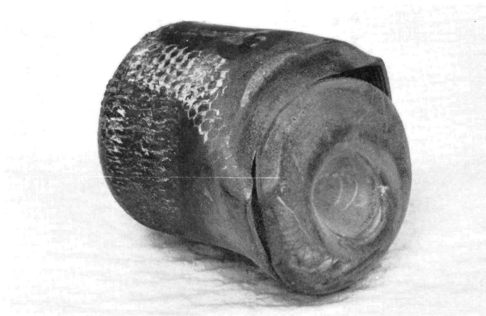
Figure 16. Recovered capsule from Impact Test I
