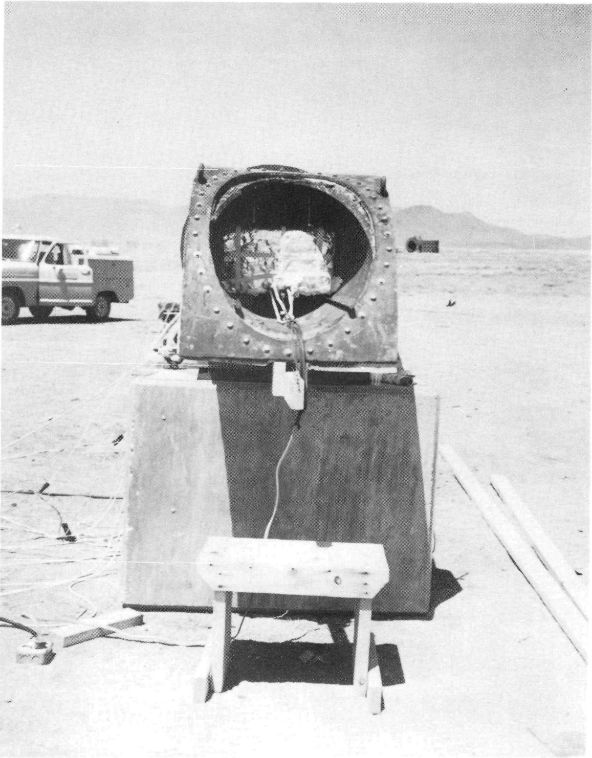
Figure 5. End view of shock tube with furnace in place
