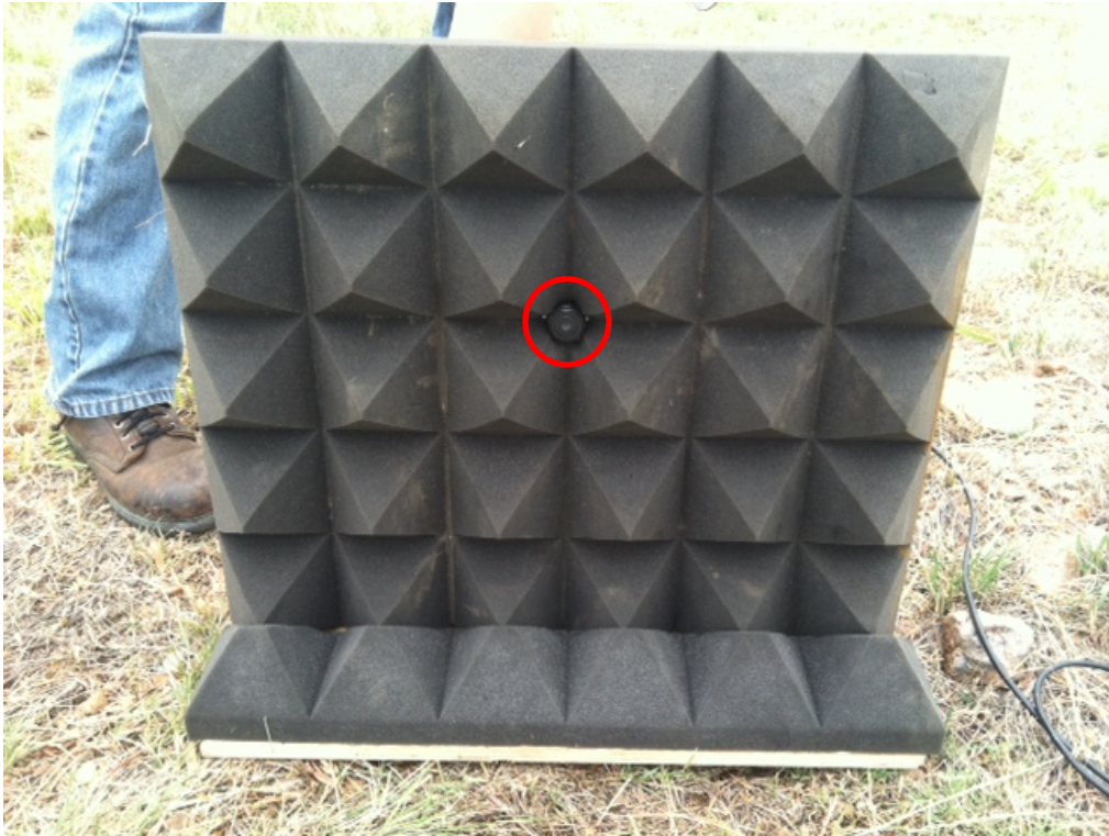
Figure 9. Isolated point source design. The speaker circled in red emits a 3.5-kHz pure tone. (Photo by Steve Buck, University of Colorado Boulder)
