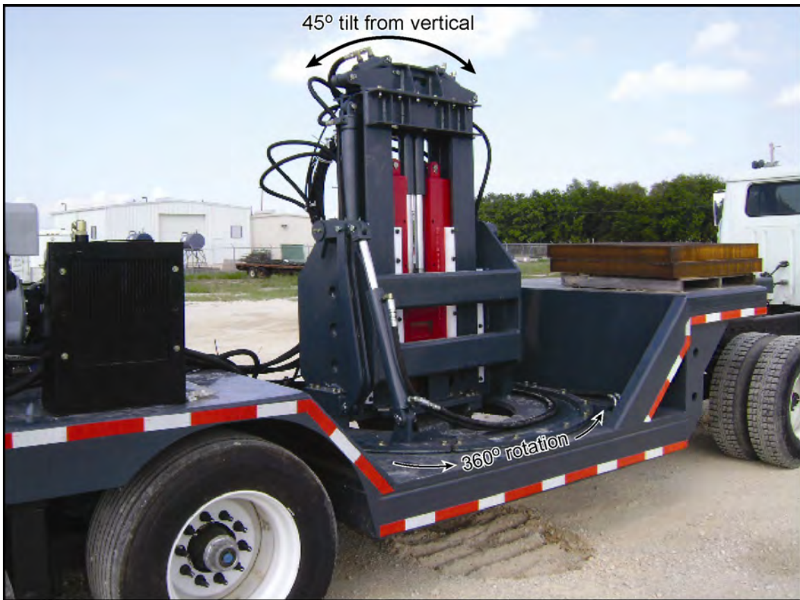
Figure 6.16. VSX™ accelerated-weight impact source provided by Vecta Technology and United Services Alliance. This source can deliver a vertical impact to the Earth, or an inclined force vector can be applied in any azimuth direction and at any incident angle between 0 and 45 degrees without moving the vehicle. Vehicle weight is 33,000 lb. Its compressed-nitrogen spring system delivers 22,276 ft-lb (30,202 joules) of energy to the Earth.
