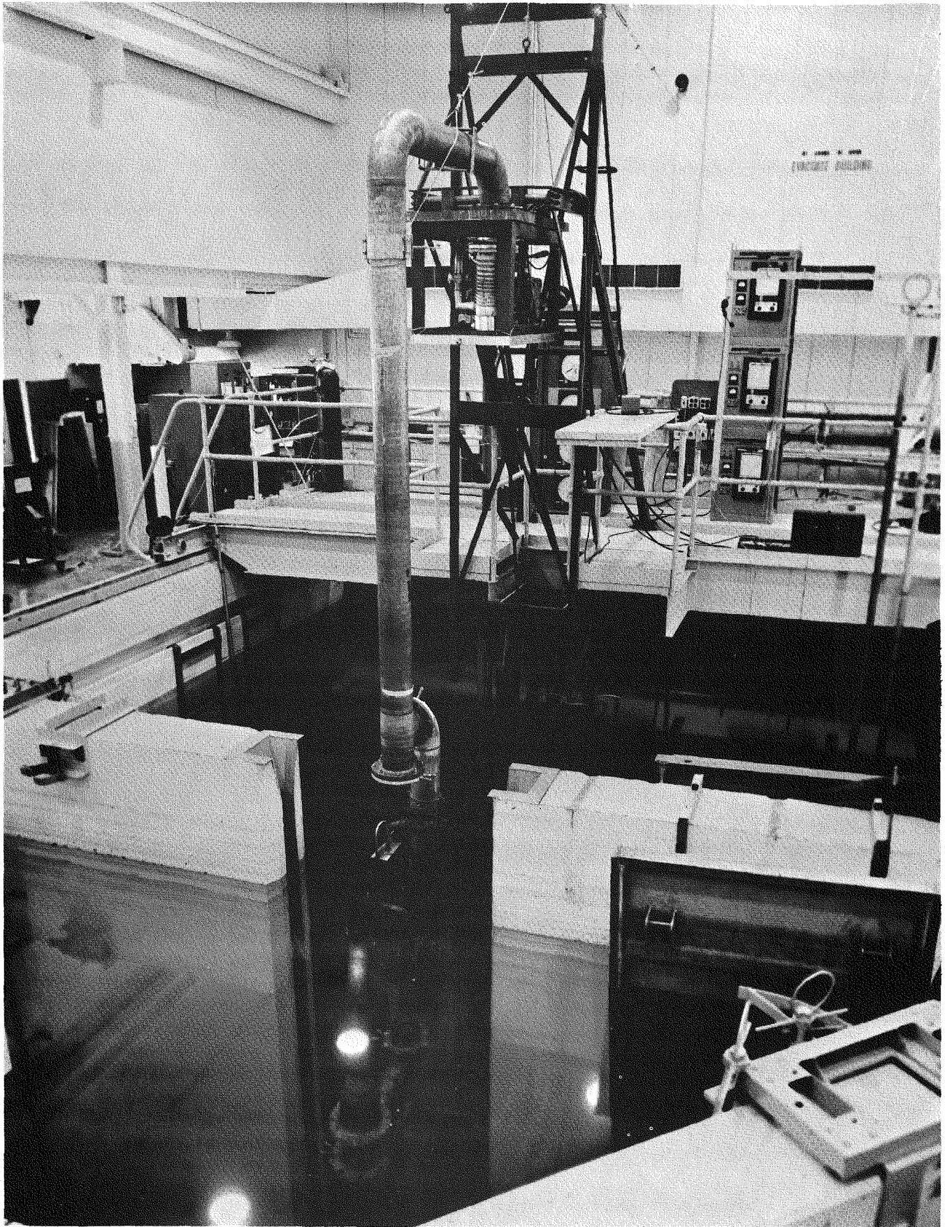
FIGURE 2. INSTRUMENT BRIDGE AND SUPPORT STRUCTURE FOR VACUUM FACILITY
