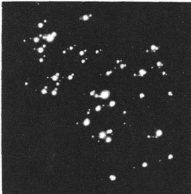
Figure 5. Autoradiograph of ^{238}\text{PuO}_2 debris from pyrocarbon coated microsphere (D68-11030)
