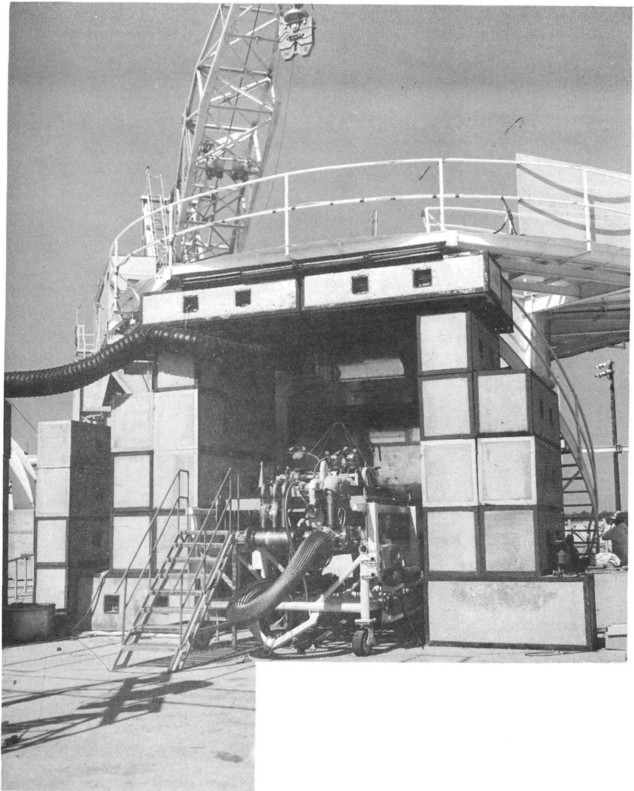
View Showing Test Pallet in Place within ASTR Outside Test Cell
