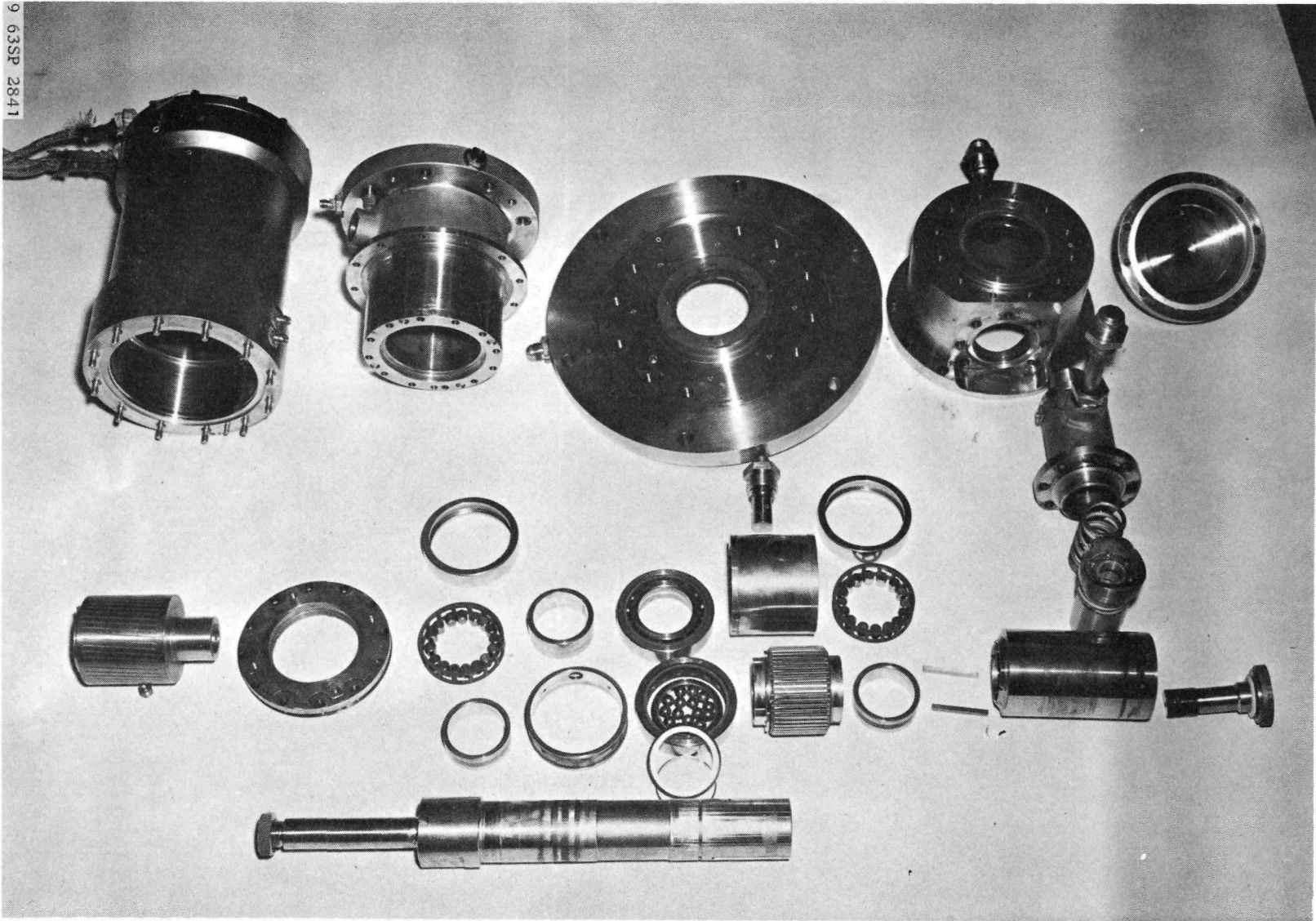
Bearing Tester PN 263500-69, SN 0000004 Disassembled after Irradiation Test (Motor to the Left; Loading Devices to the Right)
