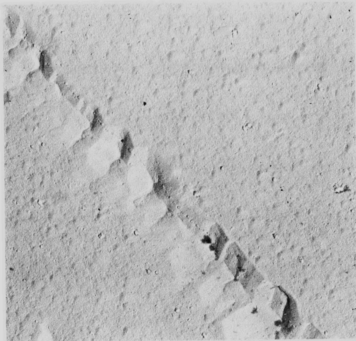
FIGURE 10. ELECTRON MICROGRAPH OF TANTALUM-4.24 a/o NITROGEN SPECIMEN ANNEALED AT 1500 C
