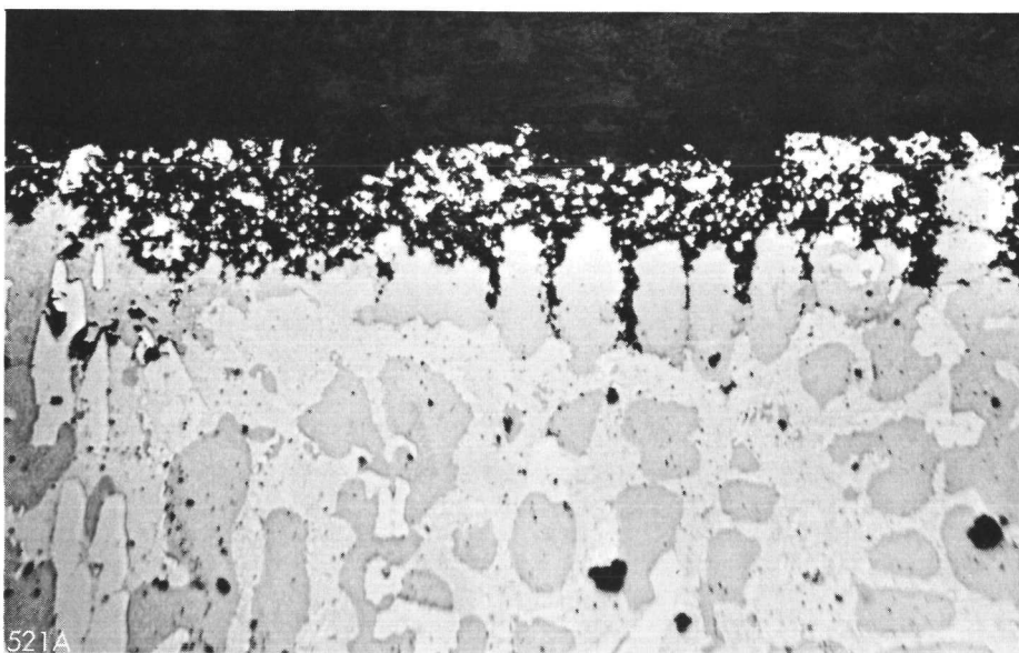
CROSS SECTION OF NICKEL-BASE ALLOY TP3 AFTER 32 DAYS IN THE BENT REFLUX TUBE AT 900°F.
