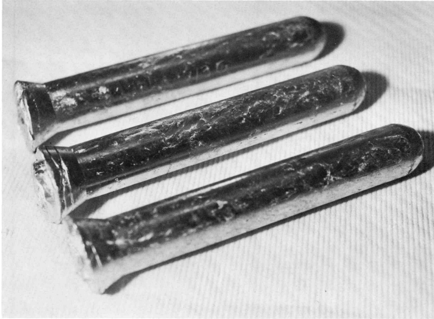
FIGURE 6 Aluminum-7.35 w/o Plutonium Alloy Fuel Core Castings (1/2X)
