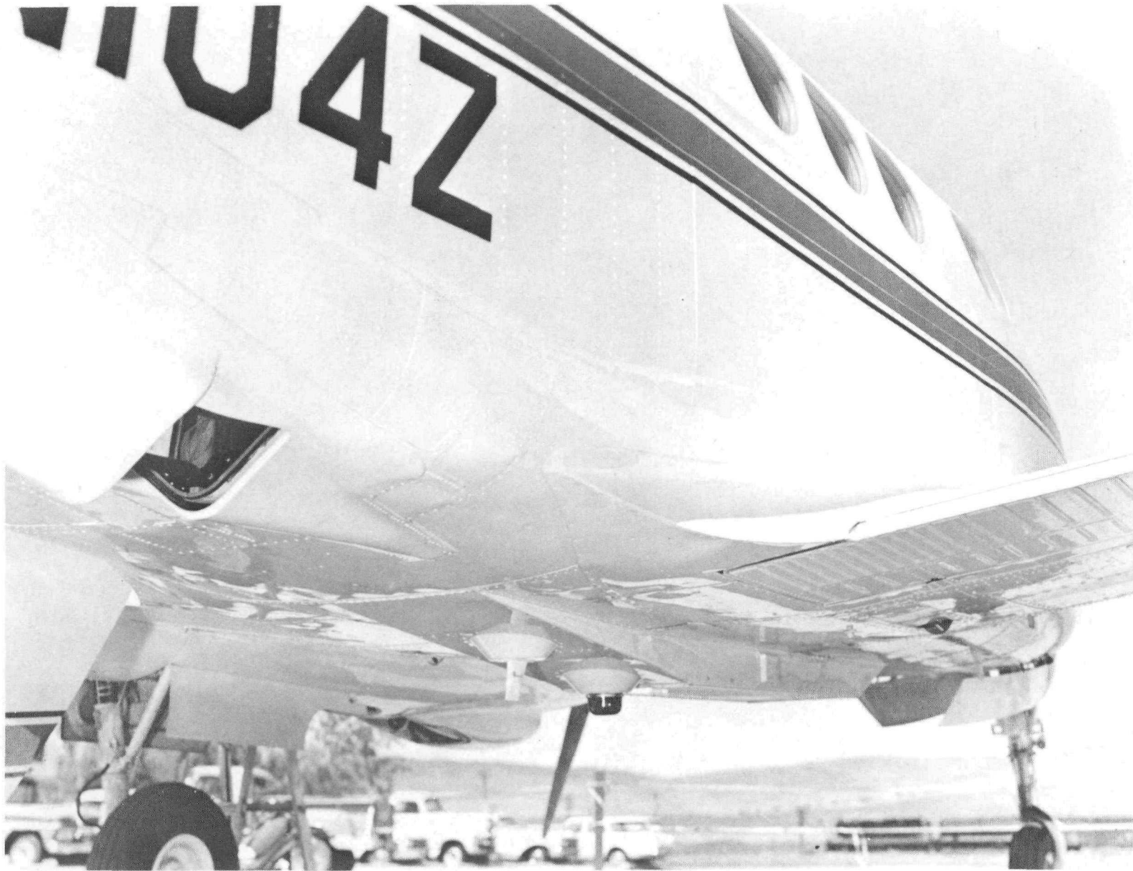
Figure 4. Close-up of infrared "window" in belly of U. S. Forest Service Project Firescan aircraft
