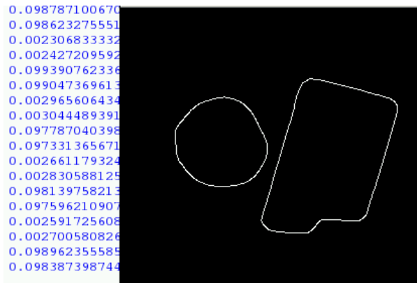
Figure 25 Illustration of shape recognition. The data (blue number) are the shape ratios of contours of blocks to a circle.
