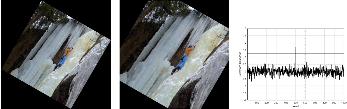
(a) Watermarked image with 30° rotation (b) Watermarked image with 30° rotation, cropping) (c) Detector's Response ( \alpha=0.65 , 30° rotation, cropping)
