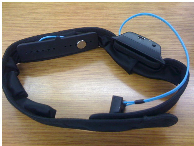
FIGURE 2.4. Example of a single electrode consumer device used for EEG recording [96].
