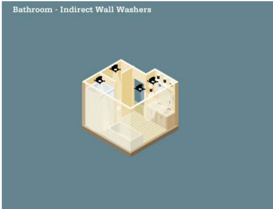
Figure 76. Indirect - wall washers.
