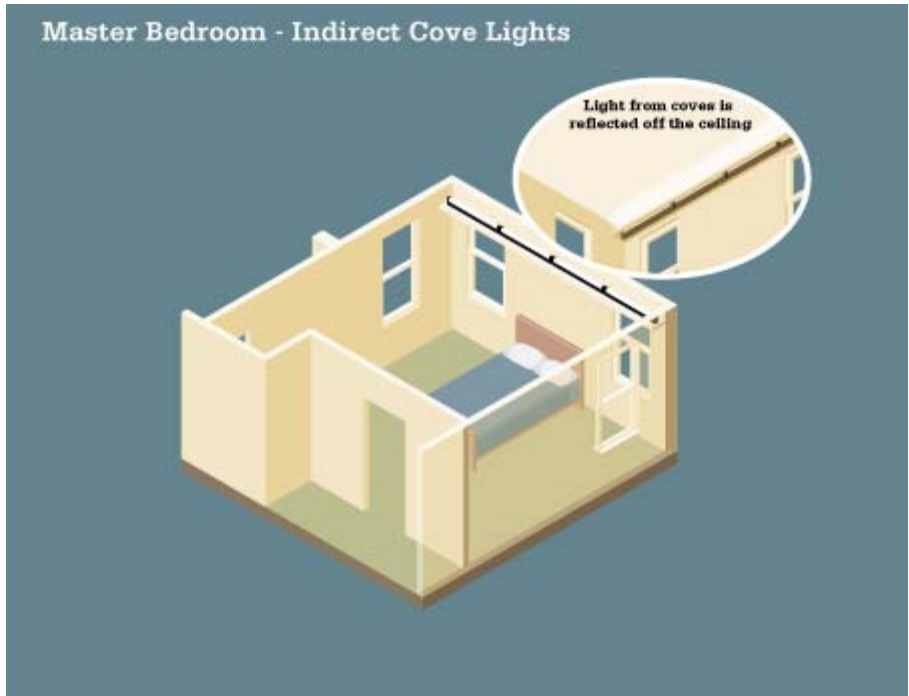
Figure 60. Indirect - cove lights. Light cove, T-5 or T-8 strip lights, continuous.
