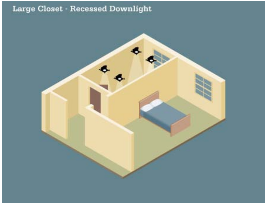
Figure 84. Recessed downlights. Recessed downlights with clear reflectors, large closet.
