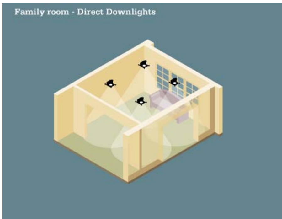
Figure 47. Direct - downlights. Recessed downlights with white reflectors.
