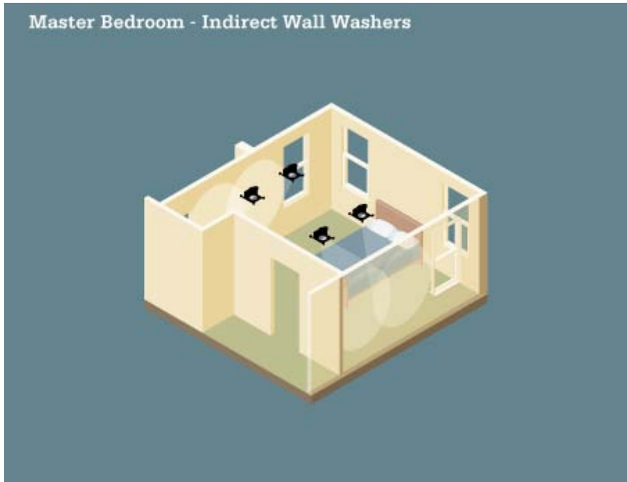
Figure 61. Indirect - wall washers.
