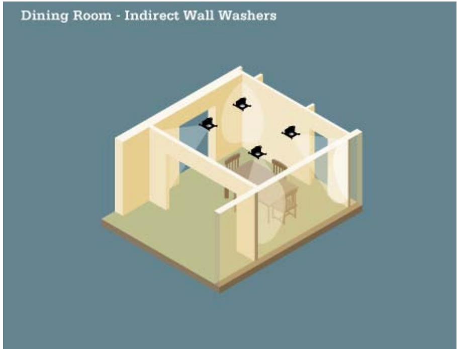
Figure 68. Indirect - wall washers.
