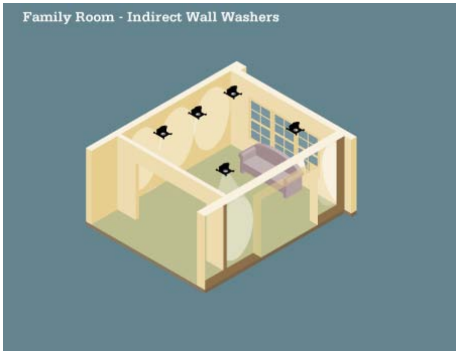
Figure 49. Indirect - wall washers.
