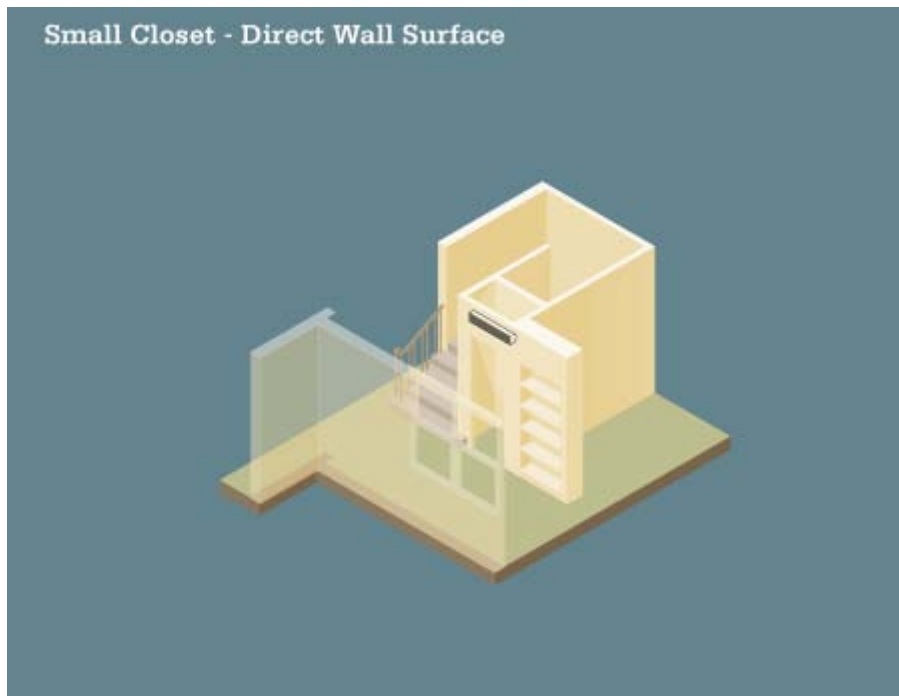
Figure 79. Direct – wall surface light. One under-cabinet light, small closet.
