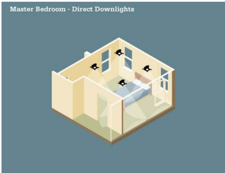
Figure 58. Direct - downlights. Recessed downlights with white reflectors.
