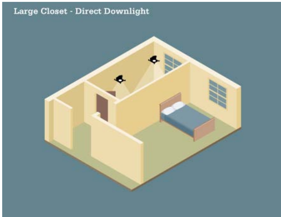
Figure 82. Direct - downlights. Recessed downlights with white reflectors, large closet.
