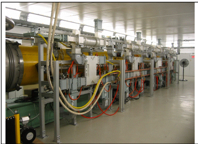
Figure 1: View of CM-1 from upstream to downstream with the waveguide distribution installed.
