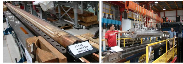
Figure 14: 4-m long Nb 3 Sn dipole coil (left) and LM02 cold mass (right).
